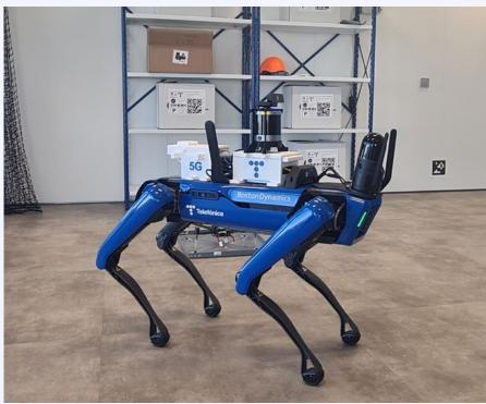
We want to help industry to automate its processes, using the latest technology with a dual purpose: optimise resources and reduce risks to workers. Our 5G network provides the ultra-high bandwidth needed to transmit a massive LiDAR point cloud (360,000 points per second) simultaneously with video streams, used as the basis for artificial vision solutions. This technology ensures a highly reliable connection, essential in critical environments.
